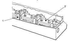
2. Ink cartridge holder plate - There are four holder plates which hold the two ink cartridges each
